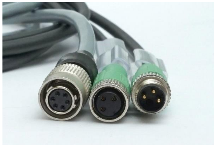
Fig. 3 – Cable connectors: from left Hirose connector for camera connection, M8 female for illuminator and M8 male for power supply
