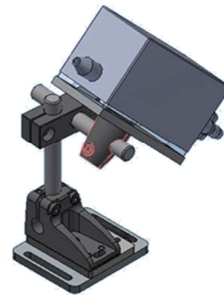
Fig. 8 – Recommended design of the detection probe attachment
