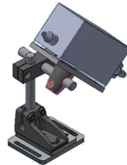
Fig. 8 – Recommended design of the detection probe attachment
