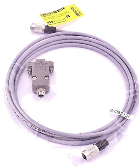
Fig. 18 – Cable for connecting PC to the control unit (PSKLAK9300), extension cable with BINDER connectors (4 pins) and with reduction to RS232 serial interface (CANNON 9pin)
